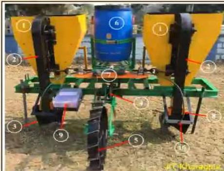
(1) Hopper, (2) Bud metering unit, (3) Furrow opener, (4) Power Transmission system (5) Ground wheel, (6) Fungicide tank, (7) Pump & solenoid valves, (8) Optical sensors, (9) Control unit and (10) Spray nozzle
