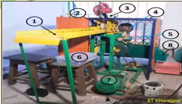
(1) Feeding chute, (2) feed rollers, (3) camera, (4) cutting arm assembly, (5) cranking motor, (6) electronic controller, (7) AC motor and (8) hood gallery
